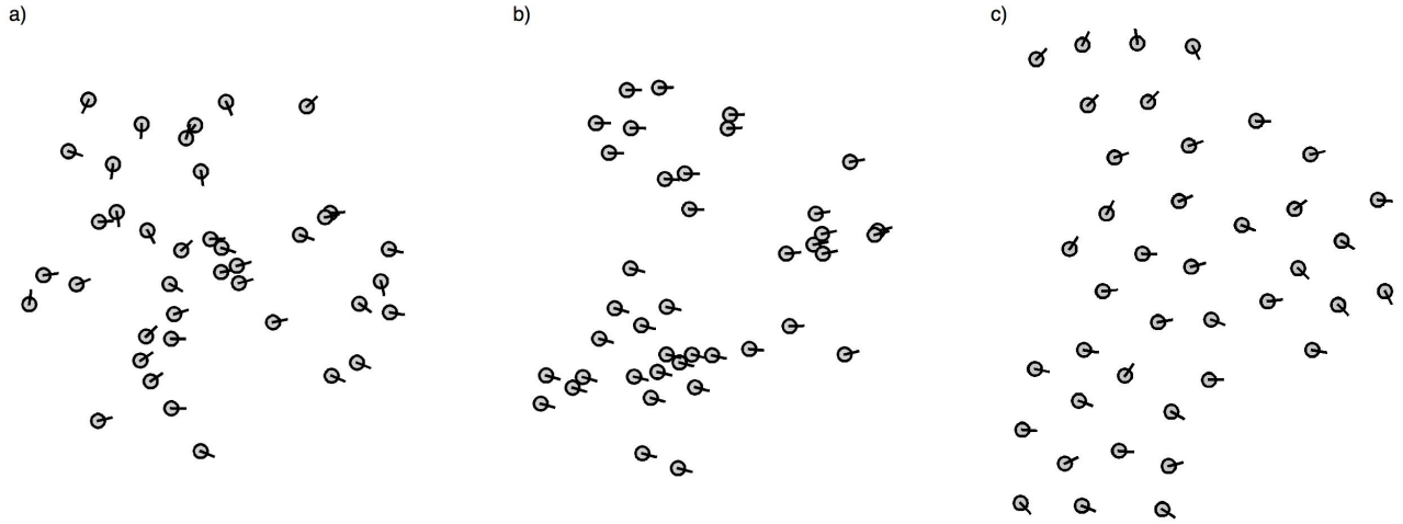
Fig. 2. Shows the swarm in each of the three possible states. After the user issues a heading command, each robot begins to move in that direction; however, before the reach consensus, the Gaussian heading error means they will not all be moving the same direction (a). After enough rounds of the consensus algorithm, the robots have all converged on an approximately identical heading (b). Finally, after the user issues the flocking constraints, the robots attempt to stay between 1.5 and 3m of each other, and thus cover more area (c).
